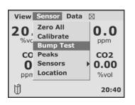
The screen to alert the user to apply gas to the instrument is then shown. The user has a fixed number of seconds to apply gas and select "Start" before the
