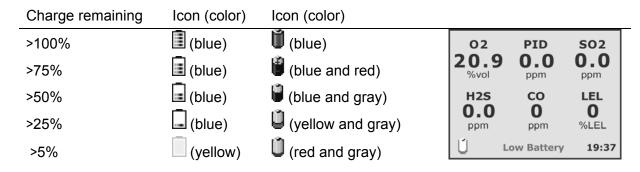
**NOTE:** If the battery life remaining is less than one hour, the battery icon flashes on the display and has an audible battery low alarm. If the run time is less than 10 minutes, the instrument alerts the user of impending shutdown by showing "Low Battery" on the lower central part of the display.
