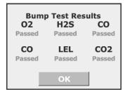
If all the sensors have passed the bump test, the instrument goes to the gasmonitoring display screen. If any sensor failed the bump test, after viewing and acknowledging the results, the instrument asks the user to continue, or calibrate the failed sensor(s). If the user selects the Cancel button, the sensor is not calibrated and the instrument moves on to the next sensor in the list. If the user selects "OK", the failed sensor is calibrated.
