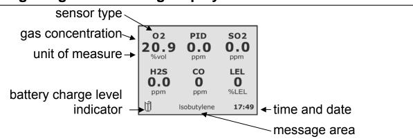
NOTE: The sample gas monitoring display screen is shown here in numeric format. Depending on the unit's configuration, some items may not display or may display differently.
