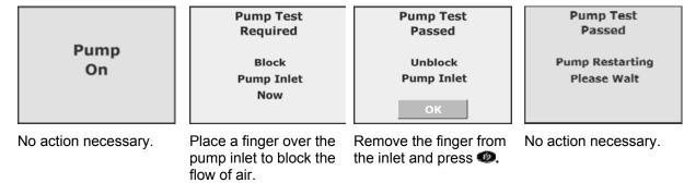
After a successful pump check, the gas-monitoring display screen is activated.
