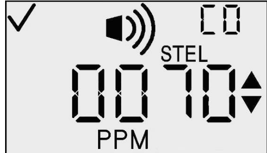
STEL Alarm Setpoint Setup
