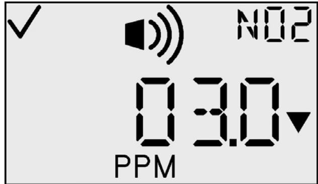
Low Alarm Setpoint Screen
