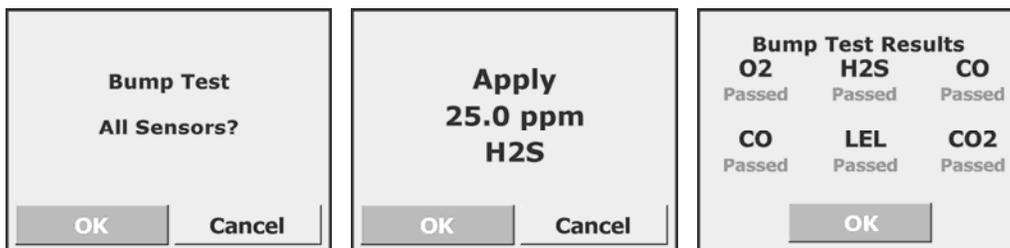
If all the sensors have passed the bump test, the instrument goes to the gas-monitoring display screen. If any sensor failed the bump test, after viewing and acknowledging the results, the instrument asks the user to continue, or calibrate the failed sensor(s). If the user selects the Cancel button, the sensor is not calibrated and the instrument moves on to the next sensor in the list. If the user selects “OK”, the failed sensor is calibrated.
