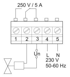
b) Connection of alarm horn or flashlight (or both)
