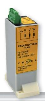
The Z-500/P device is designed for use in ungrounded networks with a nominal voltage of 500V, where the power conductors are interconnected via a consumer (e.g. an electric motor winding). The Z-500/P device, together with the ZZS-500/P device, is intended for checking the insulation resistance of individual short cable branches, namely before they are connected to the power source (deenergized).
